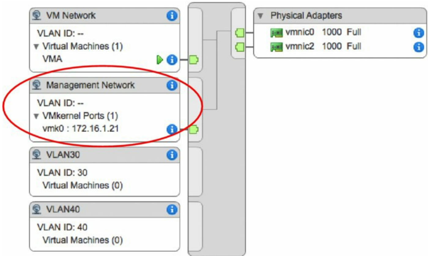
Figure 5.4 You can create virtual switches with both connection types on the same switch.
