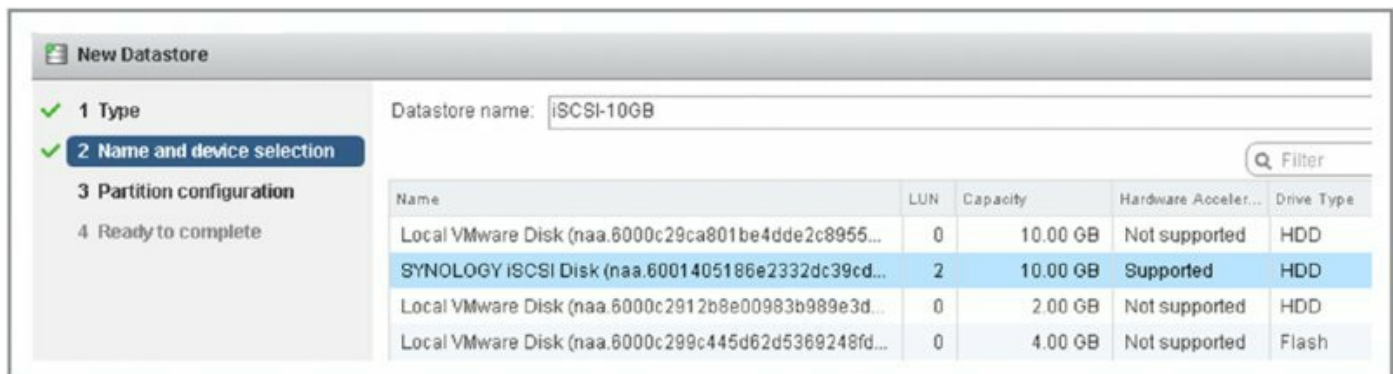
Figure 6.35 You'll choose from a list of available LUNs when creating a new VMFS datastore.
