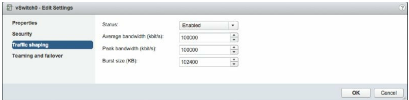
Figure 5.41 Traffic shaping reduces the outbound (or egress) bandwidth available to a port group.
