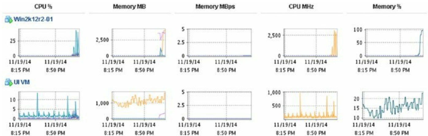
Figure 13.9 The Virtual Machines view of the Performance tab for an ESXi host in Overview layout offers both per-VM and summary information.
