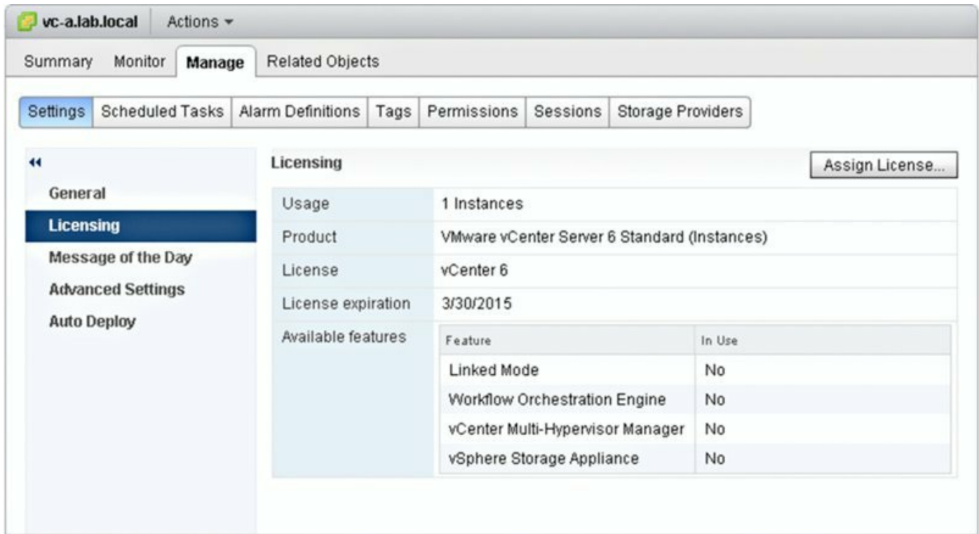
Figure 3.32 Licensing vCenter Server is managed through the vCenter Server Settings dialog box.
