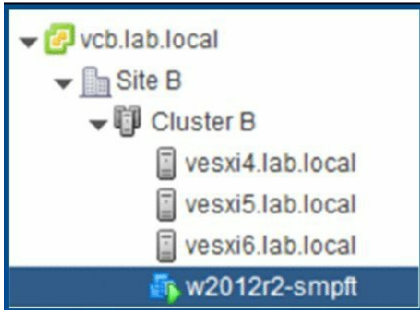
Figure 7.32 The darker VM icon indicates that vSphere SMP-FT is enabled for this VM.
